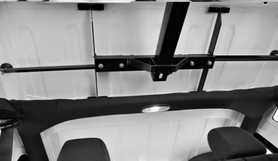
Make certain that all bolts are out of top before lifting. Recommended that no doors loaded on the Freedom Jack when pulling top as the passenger doors will hit rear door gate.
