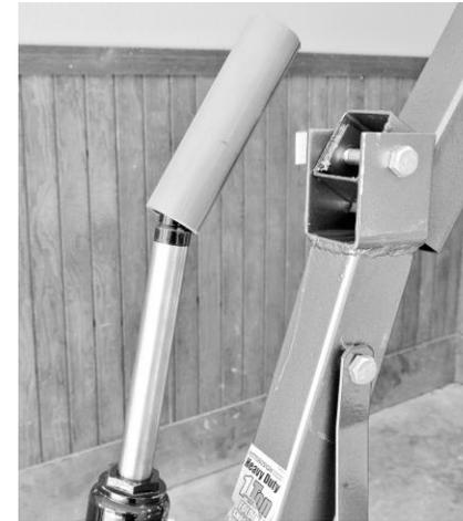
. Set up shop crane starting with sch 60 pvc tube (jack stop) provided. Take out the upper jack bolt, then slide sch 60 pvc tube over end of jack ram. If supplied with an additional jack stop angle iron place it in as you put the upper jack jack ram bolt back thru ram and boom. **Note: If you have door perch set preassembled door perch in place at this time.**
