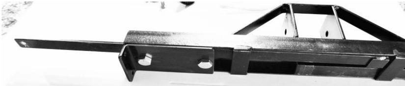
the single hole to outside of frame and facing toward top. Set lifting leg mounts on top with 90 deg. bend facing up. Put in all (4) ½" bolts that will divide extensions, put on nuts finger tight. Position LL mounts flush to main frame sides and torque nuts DO NOT OVER TIGHTEN. Fasten lift legs to LL mounts with 5/16" bolts and nuts finger tight
