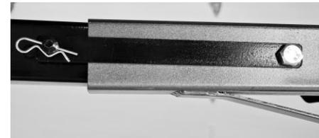
Mount Freedom Jack assembly onto shop crane using supplied 9/16 steel pin and retaining clip FJ85. **Notice:** welded on U shaped support faces rear of shop crane.
