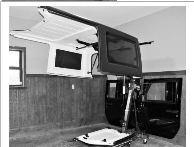
Raise top after jack has been rolled into position.
