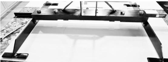
Set up on level surface where all 4 lifting leg pads are touching torque all (4) 5/16 x 1" bolts
